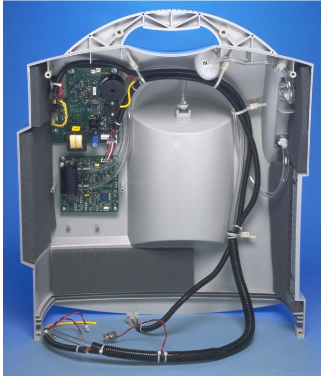
FIGURE 1: PRESSURE TUBING CONNECTIONS
