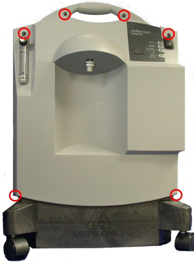
FIGURE E: FRONT CABINET SCREW LOCATION
