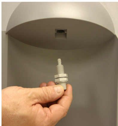
FIGURE I: REMOVING THE DISS FITTING
