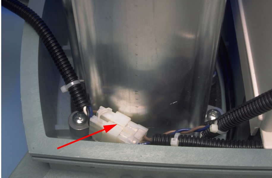
FIGURE AH: MAIN POWER WIRING HARNESS CONNECTED TO THE POWER SWITCH WIRING HARNESS
