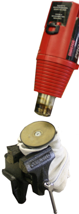
FIGURE AB: HEATING THE SCREW
