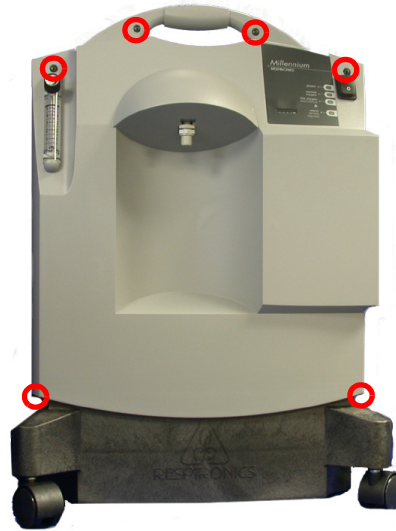
FIGURE R: SCREW LOCATIONS
