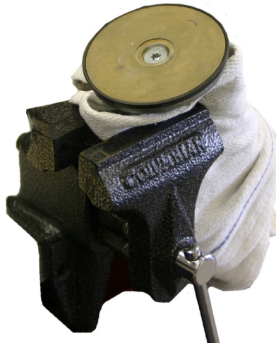
FIGURE AA: CONNECTING ROD ASSEMBLY IN VICE
