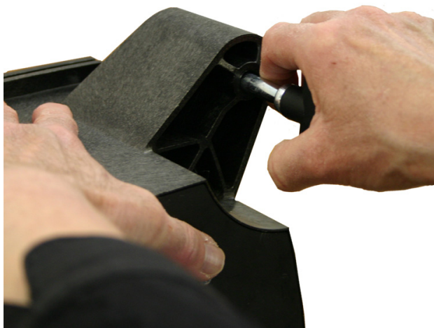
FIGURE B: REMOVING THE CASTER
