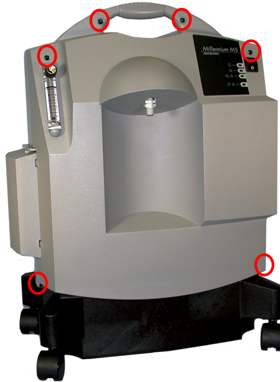
FIGURE E: FRONT CABINET SCREW LOCATIONS
