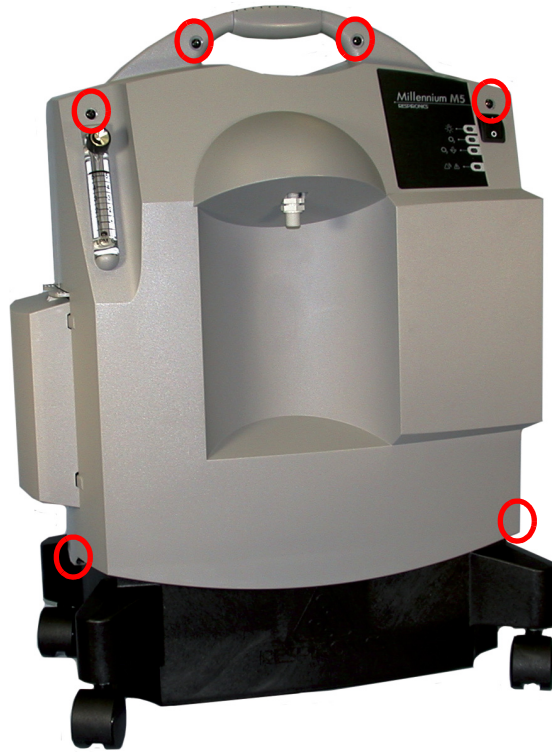
FIGURE W: FRONT CABINET SCREW LOCATIONS
