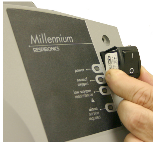
FIGURE K: REMOVAL OF THE POWER SWITCH
