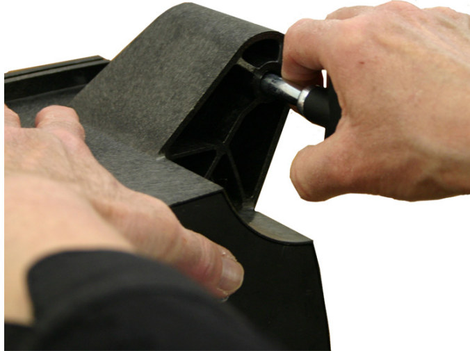
FIGURE B: CASTER REMOVAL
