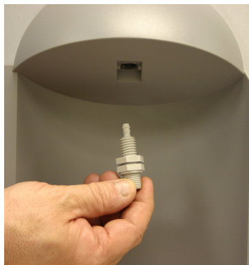
FIGURE I: DISS FITTING REMOVAL
