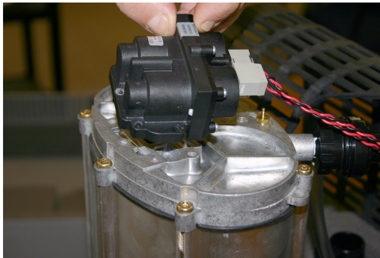
FIGURE AI: REMOVAL OF THE VALVE/SOLENOID
