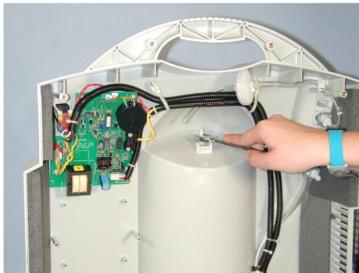
FIGURE J: REMOVE JAM NUT
