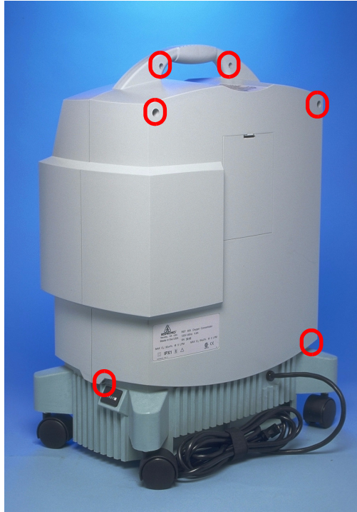
FIGURE AB: REAR CABINET SCREW LOCATIONS
