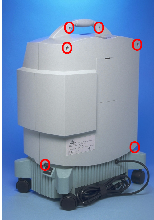
FIGURE E: REAR CABINET SCREW LOCATIONS
