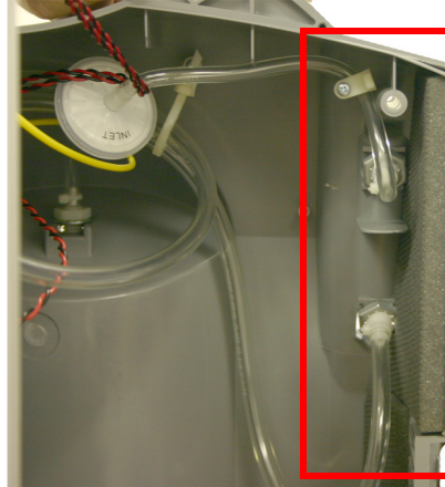
FIGURE G: VIEW OF FLOW METER FROM INSIDE THE FRONT CABINET
