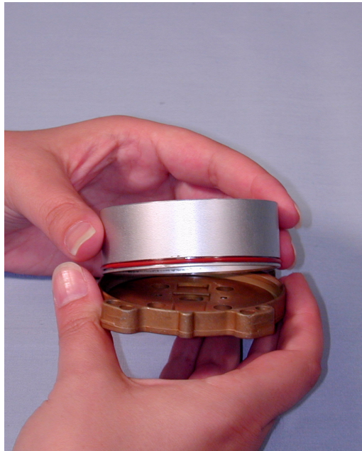
FIGURE J: SEPARATING THE CYLINDER SLEEVE AND VALVE PLATE
