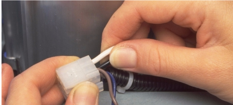
FIGURE AP: REMOVING THE POWER CORD WIRES FROM THE MAIN POWER WIRING HARNESS
