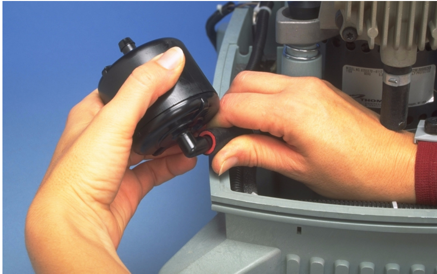
FIGURE AP: CORRECT ORIENTATION OF THE IN-LINE MUFFLER
