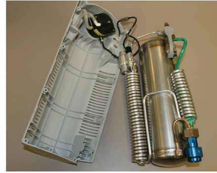
Figure 26: H850 Container Removal
