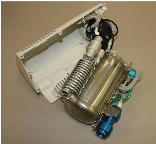
Figure 25: H300 Container Removal
