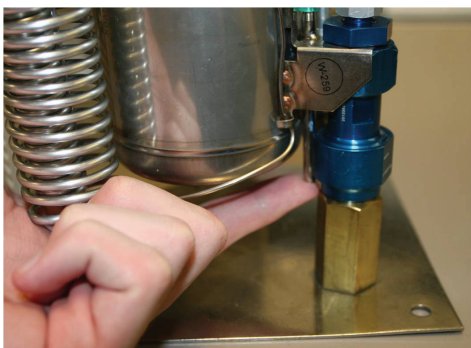
Figure 21: Vent Outlet Leak Testing
