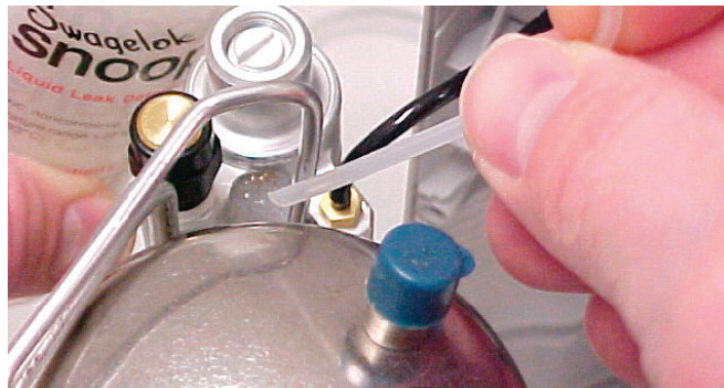
Figure 29: PRV Liquid Leak Testing
