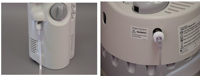
Figure 18: HELiOS Supply Line Connection
