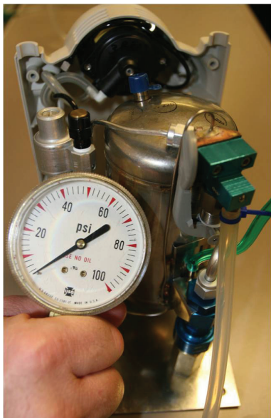
Figure 28: Test Pressure Gauge Set-Up
