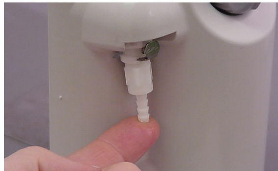
Figure 22: Inline Check Valve Leak Test
