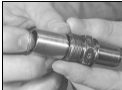
FIGURE 5-7 Inserting Retainer Ring into Male Installation Sleeve
