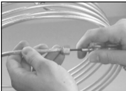
FIGURE 5-17 Straightening the Tubing
