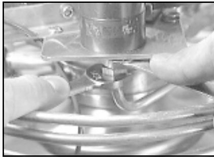
FIGURE 5-14A Removing Warming Coil from Male Connector
