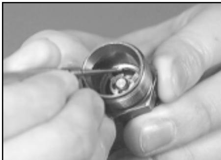
FIGURE 5-5 Removing the Retainer Ring
