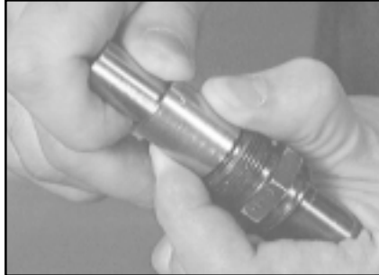
FIGURE 5-8 Reinstalling the Retainer Ring
