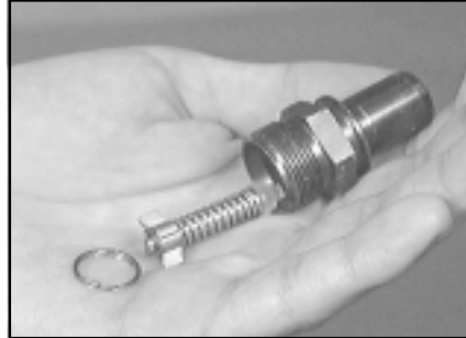
FIGURE 5-6 Removing Cartridge Assembly and Retainer Ring
