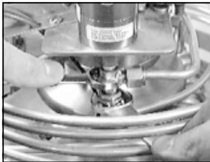
FIGURE 5-14B Removing Warming Coil from Tee
