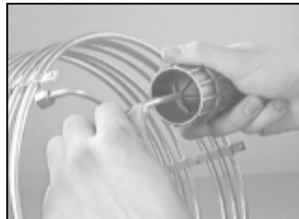
FIGURE 5-19 Deburring the Tube
